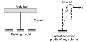
For the lateral deflection profile of the columns as shown in the figure, the natural frequency of the system for horizontal oscillation is
