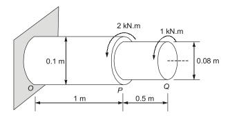
The absolute maximum shear stress in the member (in MPa, round off to one decimal place) is \_\_\_\_\_.
