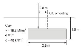
Using Meyerhoff's method, the load (in kN, round off to two decimal places) that can be applied on the footing with a factor of safety of 2.5 is \_\_\_\_\_\_.
