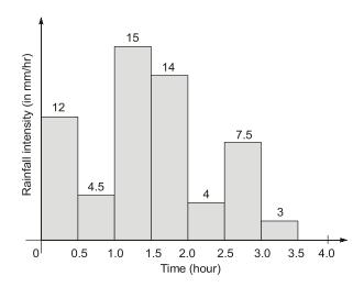
If the rainfall event has produced a direct runoff of 1.6 cm, the  $\phi$ -index of the event (in mm/hour, round off to one decimal place) would be \_\_\_\_\_.
