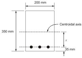
The distance of the centroidal axis from the centerline of the reinforcement (x) for the uncracked section (in mm, found off to one decimal place) is \_\_\_\_\_\_.
