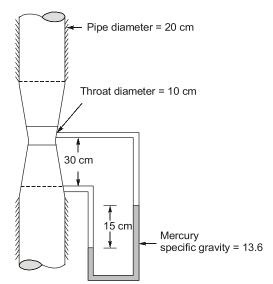
Assume  $g = 9.8 \text{ m/s}^2$ . When the deflection in the mercury manometer is 15 cm, the flow rate (in lps, round off to two decimal places) considering no loss in the venturimeter is \_\_\_\_\_\_.
