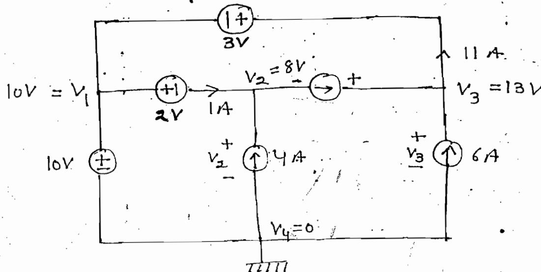
$$\text{Soln: } V_1 - V_2 = 2 \Rightarrow V_2 = 8V$$
