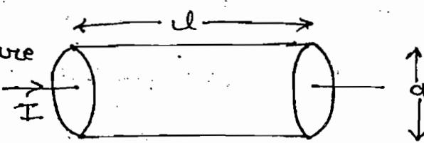
→ At constant temp. potential diff. across the element is directly proportional to current flowing into element.
