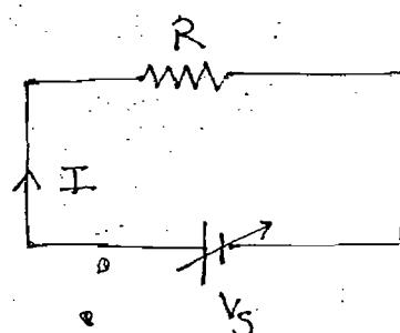
→ When element obeys ohm's law then the element is called as linear resistor
