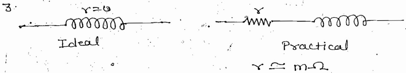
Inter-turn capacitance is present when inductor is operated at either at very high frequency or very high voltage
