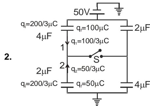
Initial and final charges are marked on  $4\mu\text{f}$  and  $2\mu\text{f}$  capacitors as shown.
