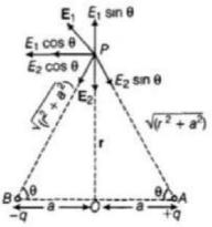
Electric field at point P due to charge -q placed at B
