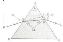
In figure, i and e are the angle of incidence and emergence respectively. Angles  $r_1$  and  $r_2$  are angle of refraction at both the surfaces of the prism. A is the angle of prism and  $\delta$  be the angle of deviation.
