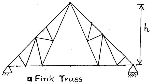
$$\text{Pitch} = \frac{\text{Rise}}{\text{Span}} = \frac{h}{L}$$
