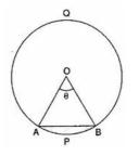
Area of segment =  $\frac{\theta}{360^{\circ}} \times \pi r^2 - \frac{1}{2}r^2\sin\theta$   $\Rightarrow$  Area of segment =  $\frac{60^{\circ}}{360^{\circ}} \times \pi r^2 - \frac{1}{2}r^2\sin60^{\circ}$   $\Rightarrow$  Area of segment =  $\frac{\pi r^2}{6} - \frac{r^2}{2} \times \frac{\sqrt{3}}{2}$  $\Rightarrow$  Area of segment =  $\left(\frac{\pi}{6} - \frac{\sqrt{3}}{4}\right)r^2$  sq. units
