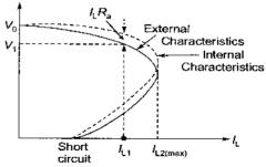
External Characteristics of DC shunt Generator
