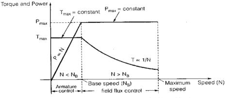
Torque and power characteristics is combined armature voltage and field control
