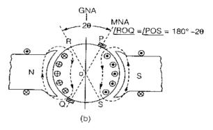
Cross magnetizing armature mmf per pole.
