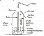
Making a soda-acid fire extinguisher.
