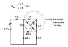
The equivalent resistance of balanced wheat stone bridge is
