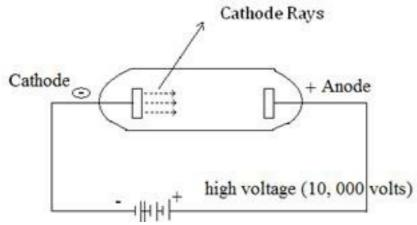
A cathode ray tube consists of two thin pieces of metals called electrodes sealed inside a glass tube with sealed ends. The glass tube is attached to a vacuum pump and the pressure inside
