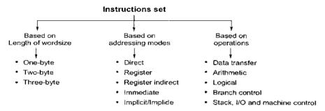
An instruction is a binary Pattern designed inside a microprocessor to perform a specific function.
