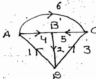
→ N/w topology is the study of the N/w properties by investigating interconnection b/w branches and nodes, it mainly concentrate on the geometry of the N/w
