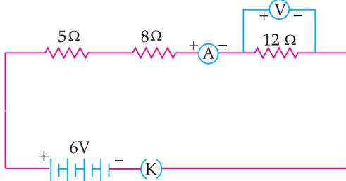
What would be the readings of the ammeter and the voltmeter when key is closed? Give reason to justify your answer.
