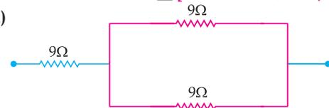
Two 9 ohm resistors in parallel connected to one 9 ohm resistor in series.
