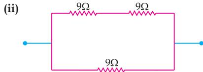
Two 9 ohm resistors in series connected to one 9 ohm resistor in parallel
