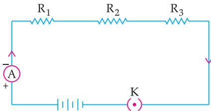
The key K is closed and the ammeter reading is recorded. Now, the position of ammeter is changed to anywhere in between the resistors. The ammeter reading is recorded each time. It is found that there is an identical reading each time, which shows that same current flows through every part of the circuit containing three resistances in series connected to a battery.
