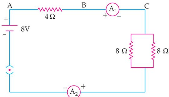
1. Effective resistance of two  $8 \Omega$  resistors in the combination.
