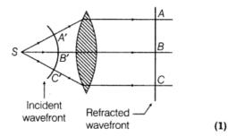
6.Sketch the shape of wave front emerging from a point source of light and also mark the rays. [Foreign 2009]
