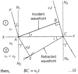
where,  $v_1$  is the velocity of light in medium 1. In the duration of time *t*, the secondary wavelets emitted from point *A* gets spread over a hemisphere of radius,
