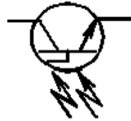
(a) IR Receiver transistor (b) Symbol of IR transistor
