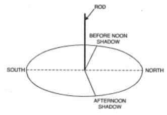
**Determining North with the help of Rod**
