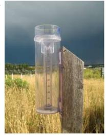
Smaller cyclinder is actually a measurement jar with milimeters, centimeters and inches marked on it. Measurement jar and the funnel have areas with specific ratio. This measurement jar is narrow cylinderical jar so that it may measure even slightest of rain water.
