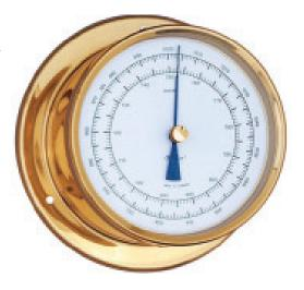
the height from the sea level. Liquids are not used in this device/it is a small round metal box in which vaccum is created.
