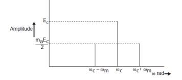
Modulation Index – the ratio of amplitude of modulating signal to the amplitude of carrier wave is called modulation index.
