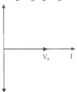
iii. A Series resonance LCR circuit is called an acceptor circuit.
