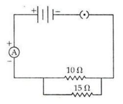
(a) State the type of combination of the two resistors in the circuit.
