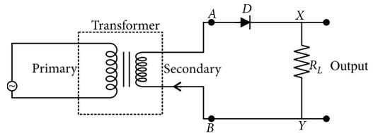
It consists of a diode  $D$  connected in series with load resistor  $R_L$  across the secondary windings of a step-down transformer. Primary of transformer is connected to a.c. supply. During positive half cycle of input a.c., end  $A$  of the secondary winding becomes positive and end  $B$  negative. Thus, diode  $D$  becomes forward biased and conducts the current through it. So, current in the circuit flows from  $A$  to  $B$  through load resistor  $R_L$ .
