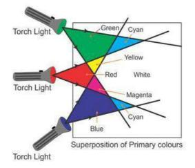
We observe that the portion of white paper where all the three patches superimpose on one another will appear white. The portions of the screen where blue and green light superimpose appear cyan. The portion of the screen where blue and red light superimpose appear magenta and it will be yellow at the superposition of red and green colours.
