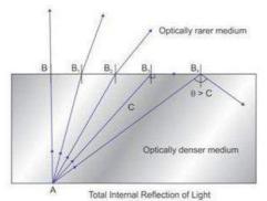
As the angle of incidence increases, the angle of refraction also increases and the ray of light moves away from normal. For a certain angle of incidence, the angle of refraction is 90°; this angle of incidence is called 'critical angle' (C). For angle of incidence greater than the critical angle ( $_{\theta > C}$ ), the light is completely reflected in the denser medium. This phenomenon is known as total internal reflection.
