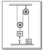
Solution: (d) Since the mass  $m_2$  travels double distance in comparison to mass  $m_1$  therefore its acceleration will be double i.e. 2a
