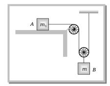
Solution: (a) When the block  $m_2$  moves downward with acceleration a, the acceleration of mass  $m_1$  will be 2a because it covers double distance in the same time in comparison to  $m_2$ .
