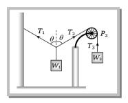
Solution: (d) Since through a single string whole system is attached so  $W_2 = T_3 = T_2 = T_1$
