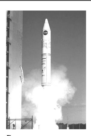
Rocket propulsion is based upon the law of conservation of linear momentum. The fuel is burnt in the ignition chamber of the rocket engine. The gases so produced are ejected from an orifice in the rear of the rocket. A thrust acts on the rocket due to reaction of the movement of gases and thus the rocket starts moving in the forward direction.
