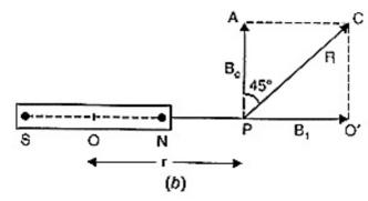
Magnetic field B<sub>2</sub> due to magnet at equatorial line
