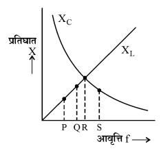
In the given figure, write a point showing the resonant state.
