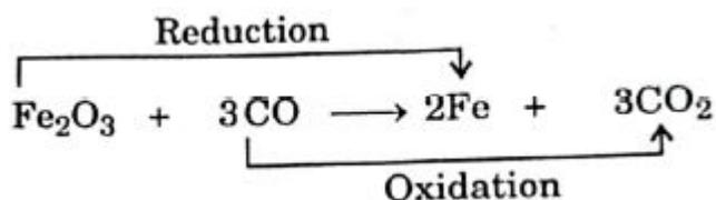
In the above reaction ferric oxide ( $\text{Fe}_2\text{O}_3$ ) is reduced into iron (Fe) by losing the oxygen atoms attached to it and carbon monoxide (CO) is oxidized into carbon dioxide ( $\text{CO}_2$ ) by gaining the oxygen atoms.
