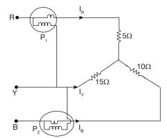
With 3-phase, 440V system of supply and the current coils of two watt meters connected in R and B phases. What will be the total load power measured by the watt meter  $P_1$  and  $P_2$ .
