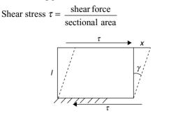
Shear stress causes an angular deformation. The change in the right angle of the element is known as shear strain. It is denoted by the angle  $\gamma$ . From the figure,
