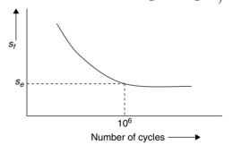
Usually  $S_f$  is taken as 0.8 to  $0.9S_u$  at  $10^3$  cycles and  $S_f = S_e$ =  $0.5S_u$  at  $10^6$  cycles for steel.  $S_e$  is further corrected using various derating factors.
