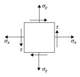
For the stresses on a small element as shown above, the principal stresses are,
