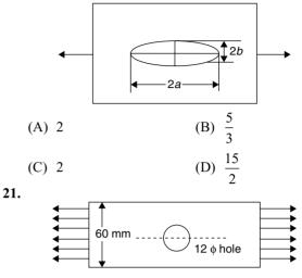
A completely reversible load of 15 kN acts on a plate with a 12 mm diameter hole as shown in figure. The plate has ultimate strength  $S_u = 440 \text{ N/mm}^2$ , notch sensitivity q = 0.8, surface finish factor = 0.67, size factor = 0.85, reliability factor for 90% reliability = 0.897. If  $k_t = 2.35$  and factor of safety = 2, determine the required minimum plate thickness in millimeter. (Take  $S_{e}' = 0.5 S_{u}$ ).
