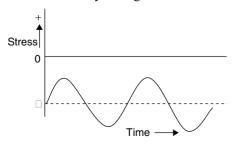
Type (3) is the general case of fluctuating stress. When the amplitude is equal in positive and negative sides as in the case (4), it is called a completely reversed stress.
