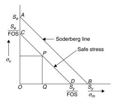
A safe stress line *CD* can be drawn parallel to *AB* taking a suitable factor of safety.
