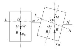
*Metacentre* (point *M*) is the point of intersection of the line passing through the centre of gravity (point G) and the original centre of buoyancy (point B) and a vertical line passing through the centre of buoyancy of the rotated position of the body (point B')
