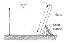
The height of the water body is such that the gate tips about the point B at which it is hinged against a solid support. If the vertical distance of the centre of pressure, on the rectan-
