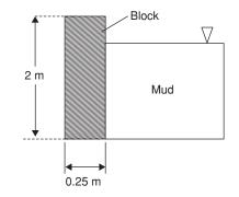
The density of concrete is  $2600 \text{ kg/m}^3$  while the density of the mud is  $1700 \text{ kg/m}^3$ . If the coefficient of friction between the ground and the concrete block is 0.4, then the mud height at which the block will start to slide is
