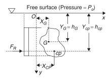
**Example 5:** For a horizontal surface of negligible thickness submerged in a fluid of constant density, let points *G* and *CP* represent the centroid and centre of pressure of the area exposed to the fluid. Then, which one of the following statement is ONLY correct about the points *G* and *CP*?
