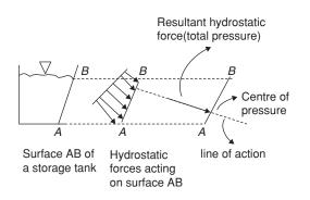
Total pressure is defined as the force exerted by a static fluid on a surface that is in contact with the fluid. The total pressure, i.e., the resultant hydrostatic force, always acts normal to the surface.
