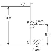
When the height of the body of liquid (present on the left side of the gate) reaches 10 m, the hinge breaks, as the reaction at the hinge becomes 1029 kN. The density of the liquid is
