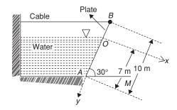
The plate is held in place, inclined at an angle of  $30^{\circ}$  to the horizontal, by a horizontal flexible cable of negligible weight attached to the plate at point *B*. If the friction in the hinge is negligible, then the tension in the cable is
