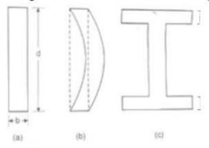
iii. A pillar with distributed ends, as shown in Fig. (b) is preferred over a pillar with rounded ends because it supports much more load than a pillar with rounded ends.
