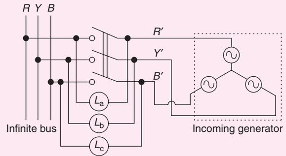
It was found that the lamps are becoming dark in the sequence  $L_a-L_b-L_c$ . It means that the phase sequence of incoming generator is [2014]
