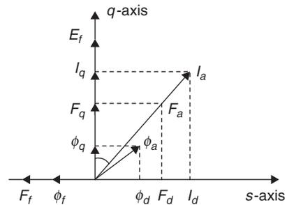
The phasor diagram of the generated voltage and terminal voltage of salient-pole synchronous machine is as shown in the following figure.
