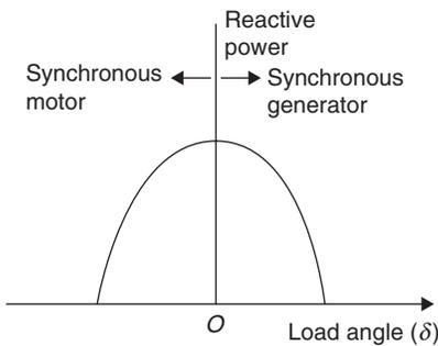
Figure 4 Reactive power versus load angle characteristic
