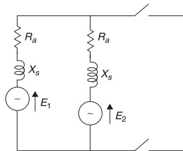
When in exact synchronism, the two alternators have equal terminal voltages and are in exact phase opposition.
