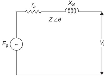
In the above circuit  $E_g$  represent the generated voltage in generator and  $V_t$  represent the terminal voltage across the generator terminals after subtracting the armature and friction drop from the generated voltage. Therefore the power input (i.e., power developed) in generator
