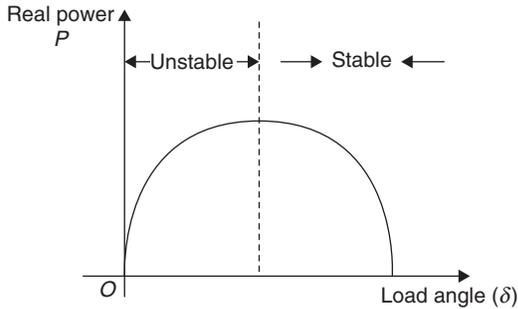
Figure 3 Real power versus load angle characteristic
