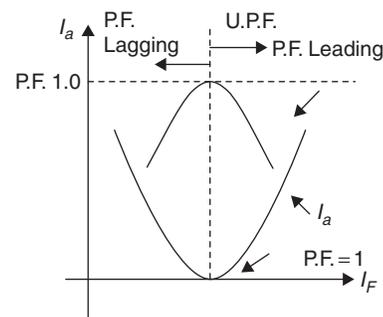
Effect of field current on an alternator connected to infinite bus is given by the V-curve and inverted V-curve shown in above figure.
