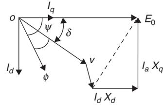
**Figure 2** Phasor diagram for a salient-pole alternator
