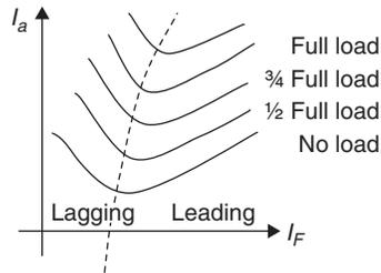
The inverted V-curves of a synchronous motor show how power factor varies with excitation (or  $I_f$ ) when motor input is constant. The curve for p.f. looks like inverted 'V' curve.
