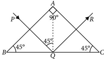
A totally reflecting prism is used to deviate the path of the ray of light through  $90^\circ$ , when it is inconvenient to view the direct light. In Michelson's method to find velocity of light, the direct light from the octagonal mirror is avoided from direct viewing by making use of totally reflecting prism.
