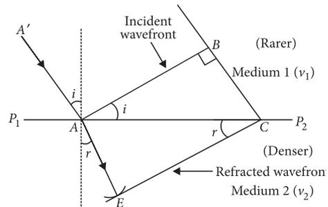
Let  $v_1$  and  $v_2$  represents the speed of light in medium 1 and medium 2 respectively. We assume a plane wavefront  $AB$  propagating in the direction  $A'A$  incident on the
