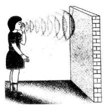
(ii) The size of the reflector must be large (like tall mountains, hills, walls, etc.) compared to the wavelength of the incident sound (for reflection of sound to take place).
