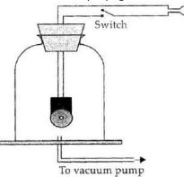
Take an electric bell, a big glass jar and vacuum pump. Hand an electric bell inside a jar connected to a vacuum pump. Switch on the bell and switch on the vacuum pump to take the air molecules out of the jar. The sound becomes feeble and finally you may not hear the sound.
