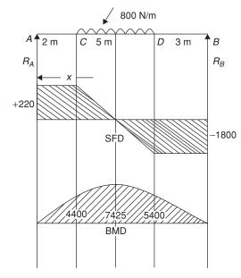
Taking moment about A  $R_B \times 10 = (800 \times 5) \times 4.5 = 1800$  N  $R_A^{\rm D} = (800 \times 5) - 1800 = 2200 \text{ N}$ Shear force at  $A = R_A = +2200$  N
