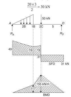
$R_A + R_D = 30 + 50 = 80$ Taking moments about A  $30 \times 2 + 50 \times 5 - R_D \times 10 = 0$
