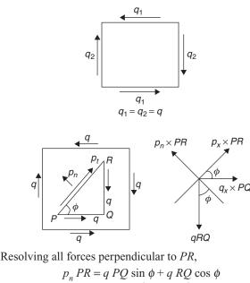
$p_n TR = q TQ \sin \phi + q RQ \cos \phi$   $p_n = q \cos \phi \sin \phi + q \sin \phi \cos \phi$   $= 2q \sin \phi \cos \phi = q \sin 2\phi$ Resolving all forces parallel to *PR*,  $p_t PR = -q PQ \cos \phi + q RQ \sin \phi$   $p_t = -q \cos^2 \phi + q \sin^2 \phi$   $= q (\sin^2 \phi - \cos^2 \phi) = -q \cos 2\phi$ When  $\phi = 45^\circ$ ,  $p_n = q \text{ and } p_t = 0.$
