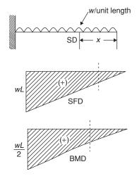
Shear force has got linear variation. F = WxBending moment varies parabolically
