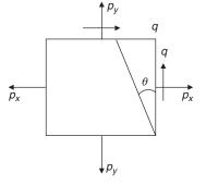
The plane makes angle  $\theta$  in the anticlockwise direction from plane at which  $p_x$  acts. As per the sign convention, radial vector will be above x-axis in positive direction.
