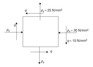
To draw the Mohr's circle first draw a horizontal line representing the normal stress and then a vertical line, representing the shearing stress. The point of intersection of these lines is the origin *O*, the point from where the stress values are plotted.
