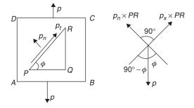
Consider a rectangular block *ABCD* subjected to the axial forces P. Consider a wedge *PQR* with angle  $\phi$  inside the block.
