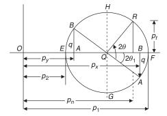
Line *AB* is the reference line representing  $p_x$ ,  $p_y$  and q. Line *QR* is drawn at an angle twice  $\theta$  (i.e.,  $2\theta$ ). Coordinates of *R* give the values of normal stress  $p_x$  and shear stress  $p_t$  on the plane.
