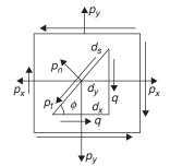
Considering a wedge of sides ds, dy and dz and unit thickness at the plane inclined at angle  $\phi$  for equilibrium,  $\Sigma F_n = 0$  and  $\Sigma F_t = 0$
