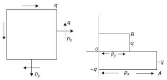
Mohr's circle is drawn on a set of axes representing normal stress (x-direction) and shear stress (y-direction).
