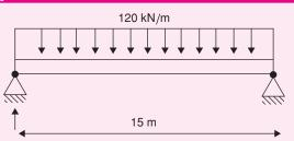
The beam is subjected to a maximum bending moment of [2004]
