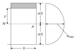
In the above expression, q, the shear stress is at a distance y from the neutral axis  $a\overline{y}$  is the moment of area above this section.
