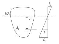
Stress is varying linearly across the depth. Consider an element area  $\delta a$  at a distance *y* from the neutral axis. Let *f* be the stress on this area.
