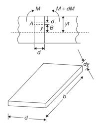
In a beam, consider an elemental length of length dx. Moments acting at the two sides of this element = M and M + dM.
