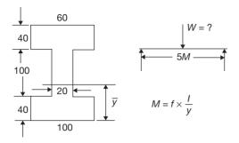
Moment carrying capacity of the beam is to be found out. For this, distance *y* from the centroid is to be found out for both tension and compression. So, position of the centroid is to be located first.
