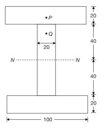
The shear stress at point P (very close to the bottom of the flange) is 12 MPa. The stress at point Q in the web (very close to the flange) is
