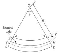
After bending, cross-sections *AC* and *BD* subtend an angle  $\theta$  at *O*. Let, *R* be the radius of the neutral plane represented by *EF*. Then, *EF* =  $R\theta$ .
