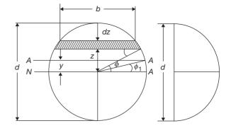
In the given circular section of diameter d, shear stress is to be determined at a section AA at a distance y from the neutral axis NA. For finding the moment of the area above AA, an element of thickness dz at a vertical distance z from neutral axis is considered.
