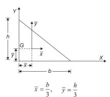
Moment of inertia about axes through G:
