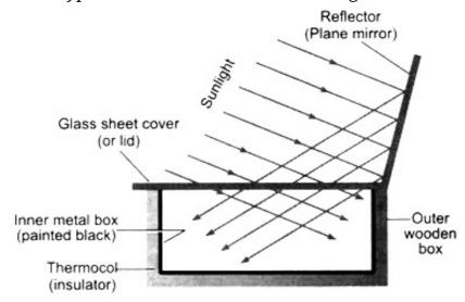
Construction of a box-type solar cooker:
