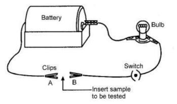
Insert the sample to be tested between clips A and B If the bulbs glows, the sample
