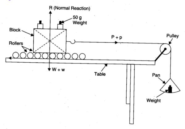
Fig. Study for force of rolling friction.
