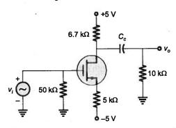
Q.14 Consider a circuit shown in figure below. The transistor parameters are
