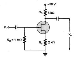
If  $g_m = 4000 \,\mu\text{U}$  then closed loop gain of amplifier is given by
