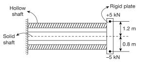
Outer radius of hollow shaft = 5 cmInner radius of hollow shaft = 4 cmRadius of solid shaft = 3 cm(A) 78.4(B) 62.4(C) 86.9(D) 72.9
