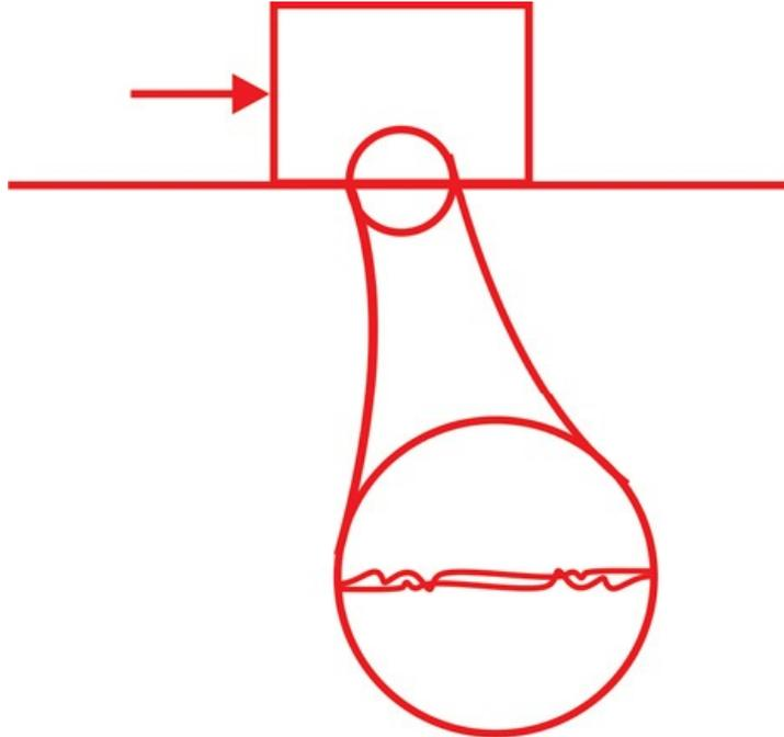
**Fig-10: Irregularities of two surfaces in contact**
