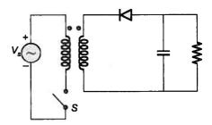
Q.16 In the following circuit. The RMS value of load current in amps by assuming  $\alpha = 90^{\circ}$  is \_\_\_\_ (in amp).
