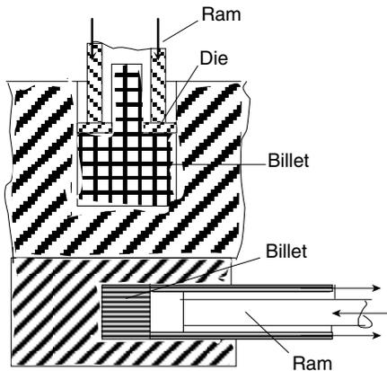
In indirect extrusion, the billet inside the cylinder has no relative motion with the cylinder. So there is no friction between cylinder and billet. Therefore power required for indirect extrusion is less compared to direct extrusion. But the long hollow ram is required and this limits the loads that can be applied.
