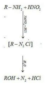
(ii) Primary aromatic amines react with nitrous acid (HNO2) in cold (273-278 K) to form diazonium salt.
