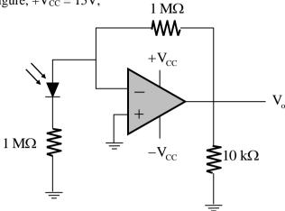
$-V_{CC} = -15V$ , Load resistor  $R_L = 10k\Omega$ . If  $10\mu W$  of power is incident on the photodiode, then the value of the photocurrent (in  $\mu A$ ) through the load is \_\_\_\_\_.
