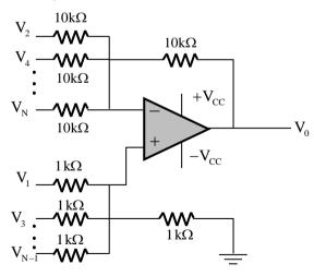
The voltages  $V_1$ ,  $V_2$ ,  $V_3$ ,  $V_4$ ,  $V_5$ ,  $V_6$ ,... are 1, -1/2, 1/3, -1/4, 1/5, -1/6,... volt, respectively. As N approaches infinity, the output voltage (in volt) is \_\_\_\_\_.
