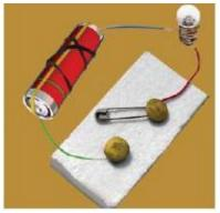
(b) Select the insulators and conductors from among the following materials: Plastic scale, rubber, aluminium foil, thermocol.
