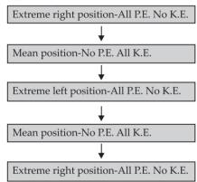
Bob eventually comes to rest due to friction of air which converts its mechanical energy into heat energy. It does not violate the law of conservation of energy has been changed from one form to another form.
