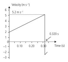
The ball has mass 0.23 kg and leaves the thrower's hand at t = 0. It hits the ground at t = 0.320 s and rebounds with 50% of the speed with which it hit the ground.
