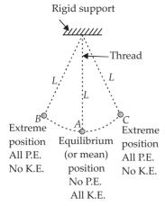
The bob of a simple pendulum swings from one extreme position to the other through its mean position.
