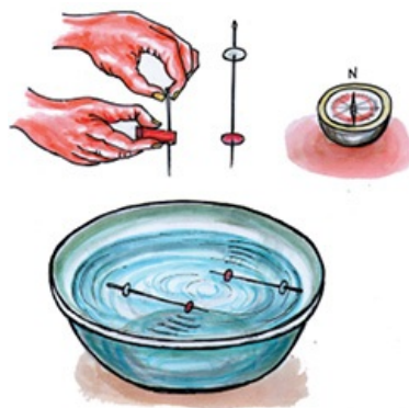
Fig-9: Making needle magnets and floating them in a bowl of water.
