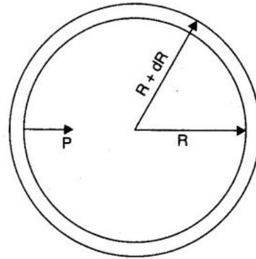
Fig. 11.01. Excess pressure inside a liquid drop.
