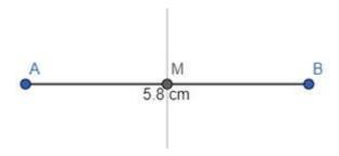
STEP 3: Then draw arcs of radius 2.9 cm from M on both the sides of the perpendicular line.
