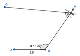
Step 5: Taking C as centre draw arc of radius 4.6 cm which cuts the segment CG. Point of intersection is D.
