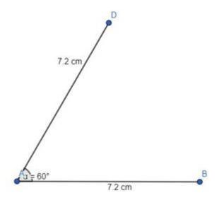
STEP 3: Now from D and B both the points, draw arcs of radius of 7.2 cm, intersecting at a same point. That point is C. Join BC and DC.
