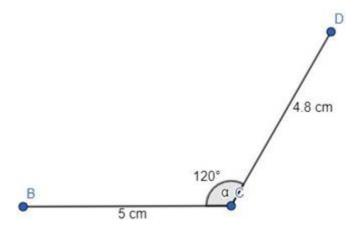
STEP 3: Now, from point B draw an arc of radius 4.8 cm and from point D draw an arc of radius 5 cm with the help of compass. The intersecting point of both the arcs is A. Join BA and DA.
