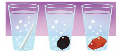
When the chalk is put in water the air comes out of the chalk in the form of bubbles. Now repeat this experiment with a mud cake and a brick.
